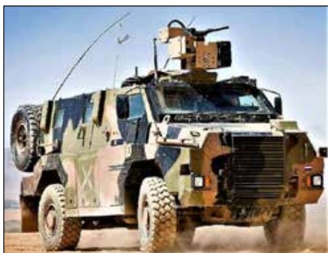
Bushmaster Protected Mobility Vehicle, an Australian design-with a V-shaped hull that provides a high degree of protection against land mines still being used successfully in Afghanistan
