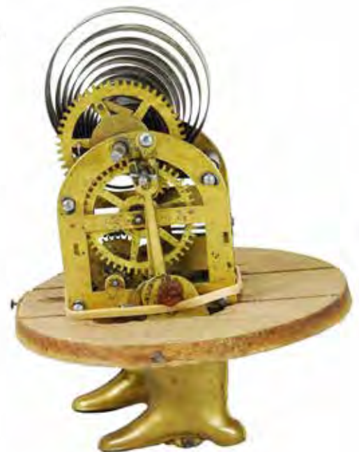
Illus. 5. The Autoperipatetikos mechanism attached to a doll's wooden base. By Courtesy of C. T. Auctioneers and Valuers Ltd.
