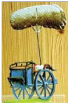
An early flat Drachen style observation balloon cabled to a hand-cranked winch mounted on a wagon attributed to Johann Haffner. The Drachen (kite or dragon) balloon was introduced by Germany in 1896. (photo courtesy of Bernhard Schwarz)
